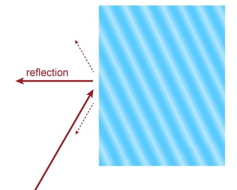
Holographic generated volume gratings, with a thickness much larger than the wavelength, often shows a narrow bandwidth around particular wavelength and angle. Following the two-beam interference exposure process, a volume grating inside fused silica is generated and simulated with the rigorous Fourier modal method (FMM) in VirtualLab. Both the spectral and angular dependent reflection property of the grating are analyzed.
